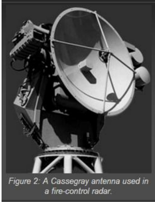
Figure 2: A Cassegrain antenna used in a fire-control radar.
