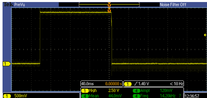
Figure 2. Button signal without a capacitor.
