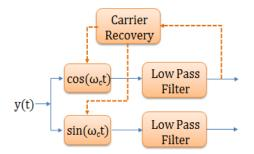
Once the in-phase and quadrature signals are separated out properly, the next task is to match each symbol with the transmitted pulse shape such that the overall SNR of the system improves.
