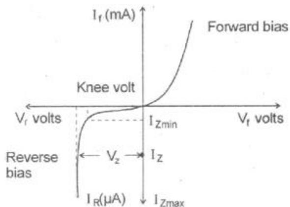
Figure 15 VI Characteristics of Zener diode
