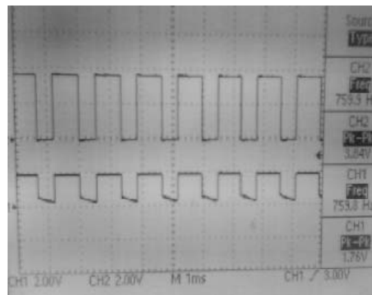
Figure 6: clock pulses and Intensity Modulated Current Driver
