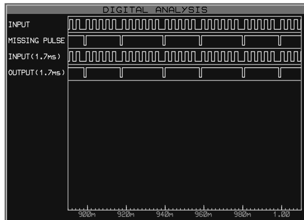
Figure 10: Output of Pulse Missing Detector.
