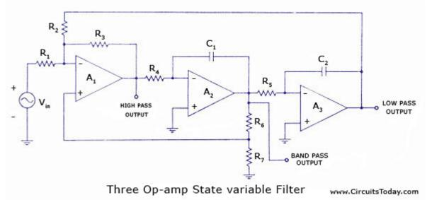
A schematic of a three op-amp, unity gain state variable filter is depicted in figure. Op-amps  $A_2$  and  $A_3$  are integrators while op-amp  $A_1$  sums the input with the low-pass output and a portion of the bandpass output. The circuit is actually a small analog computer designed to solve the differential equation (transfer function) for each filter type.
