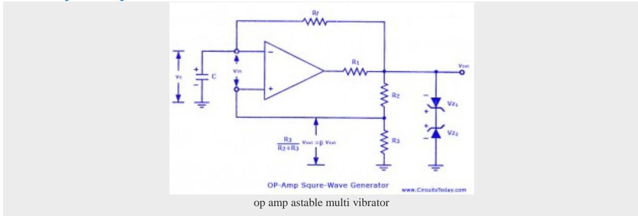
The non-sinusoidal waveform generators are also called relaxation oscillators. The op-amp relaxation oscillator shown in figure is a square wave generator. In general, square waves are relatively easy to produce. Like the **UJT relaxation oscillator**, the circuit's frequency of oscillation is dependent on the charge and discharge of a capacitor C through feedback resistor R<sub>f</sub>. The "heart" of the oscillator is an **inverting op-amp comparator**
