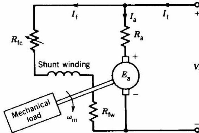
The armature current  $I_a$  and the motor speed  $\omega_m$  depend on the mechanical load connected to the motor shaft. Fig.3.30 Shunt DC motor equivalent circuit
