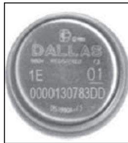
Fig.2: A typical iButton chip
