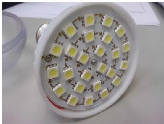
I could see its simplicity; SMD 5050 has 25 series, with an intermediate electronic transformer (wrapped in insulating plastic) that converts 220V AC to 70V DC, so each LED working at 2.8V ( $70/25 = 2.8$ ).
