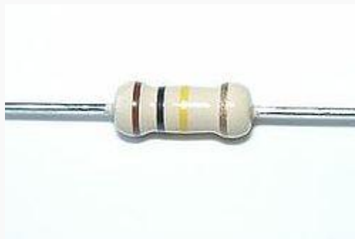
A 100 k \Omega , 5% through-hole resistor.
