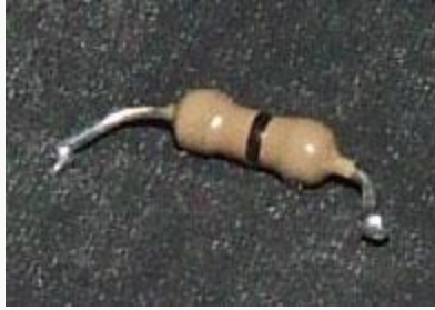
A 0Ω resistor, marked with a single black band.
