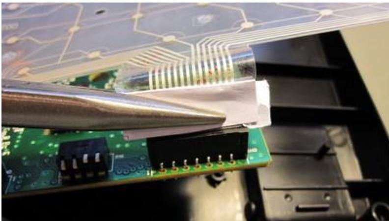
I also noticed that silver wires on the keyboard matrix itself seem to be developing a kind of a dark oxide on the outer edges. I don't remember for sure whether they looked like this from the start though. If something is eating away at the wires that definitely puts a kind of a definitive limit to this keyboard's longevity.
