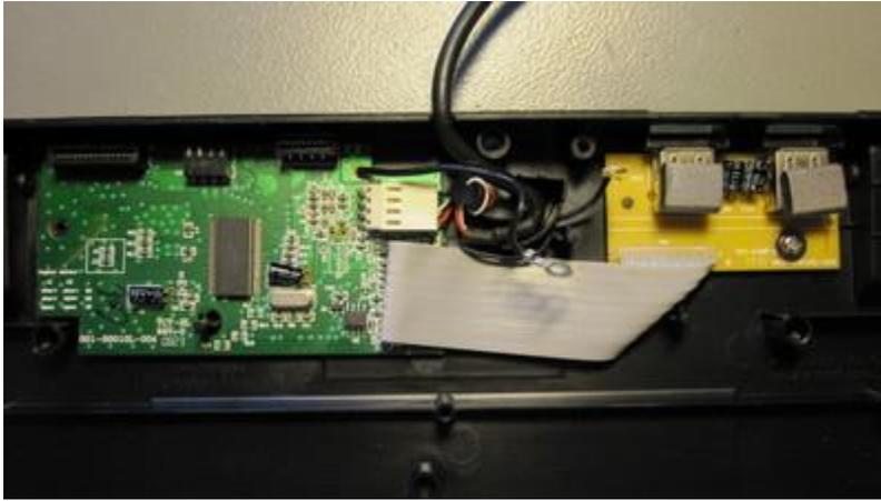
Since I had some problems with flaky USB cables before, I removed the original cable and soldered a new cable directly to the circuit board. This fixed the problem! After poking around some more, it turned out that after re-soldering the connector to the PCB the original cable worked as well.
