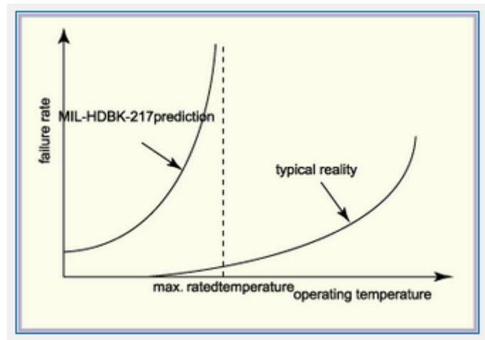
Figure 1: Failure rate plotted against temperature for electronic components
