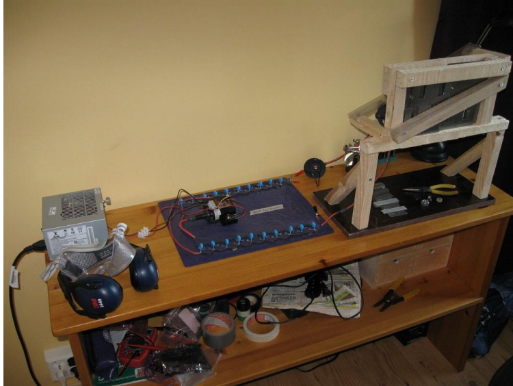
Marx generator and shielded 2X2-A rectifier.
