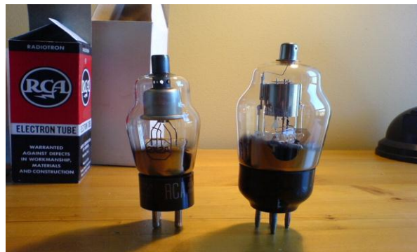
High voltage rectifier tubes. American 2X2-A on the left, and CV-1290 on the right.
