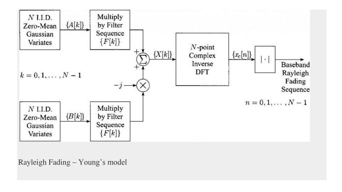
The Fading effect + Doppler Shift is simulated by multiplying the Gaussian Random variables and the Doppler Shift's Frequency domain representation. Then IDFT is performed to bring them into time domain representation. The Doppler Filter used to represent the Doppler Shift effect is derived in Young's paper.
