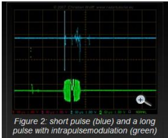
Figure 2: short pulse (blue) and a long pulse with intra pulse modulation (green)
