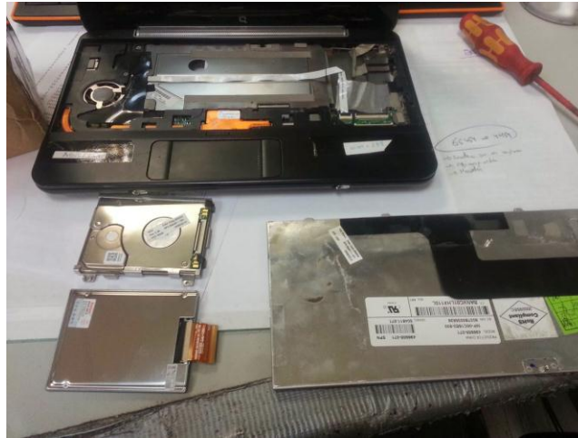
Top conventional disk 1.8 "; under SSD 1.8"
