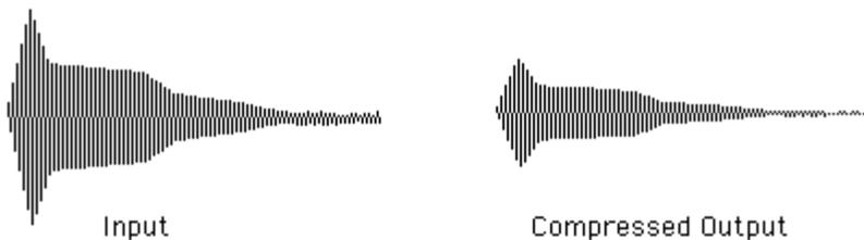
A compressor works by measuring the average amplitude of the input signal and using the information from that measurement to control the gain of an amplifier. If the measurement comes out above an adjustable threshold, the gain is reduced, if the measured input amplitude is below the threshold, the gain is increased. The amount of
