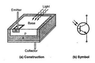
A phototransistor can be either a two lead or a three lead device. In a three lead device, the base lead is brought out so that it can be used as a conventional BJT with or without the light sensitivity feature.
