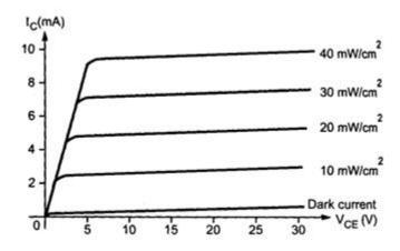
Each curve on the characteristic graph is related to specific light intensity. The collector current level increases corresponding to increase in the light intensity. In most of the applications the phototransistor is used as a two lead device. The phototransistor is not sensitive to all the light but sensitive to light within a certain range. The graph of response against wavelength is called spectral
