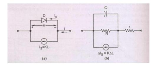
The Fig shows the small signal model for photodiode. Photodiode is represented by an ideal junction diode in parallel with a current source which is proportional to the light intensity.
