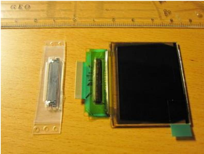
This is Densitron DD-160128FC-2B (original manufacturer's site). It's an 1.69 inch color dot-matrix display using organic LEDs on a glass substrate driven by a passive matrix. This means that you get 160 x 128 pixels with 18 bits of color resolution in a viewable area of around 36 x 29 mm (making for 110 DPI).
