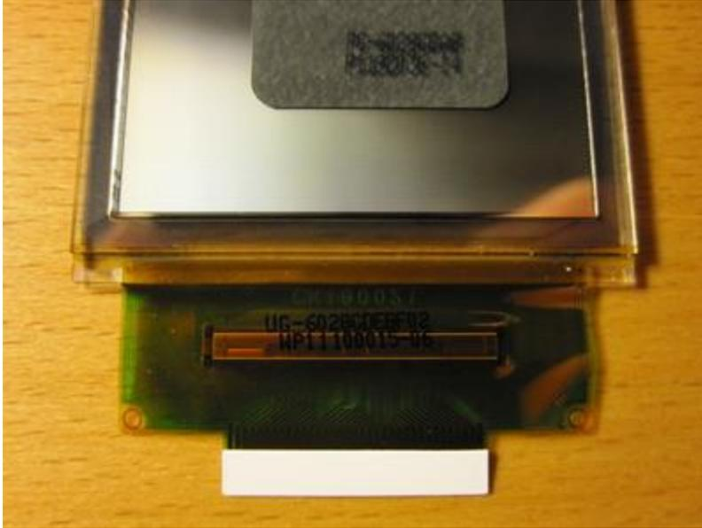
On the electronic side it's controlled by a Syncoam SEPS525 driver IC. By the way, that's the elongated bar on the front side of the display bonded to the flexible PCB tail - you can actually see the structure on the silicon through the transparent substrate. This chip supports quite a few possibilities of interconnect, although not all are usable with this particular display since some pins of the chip aren't available on the connector.
