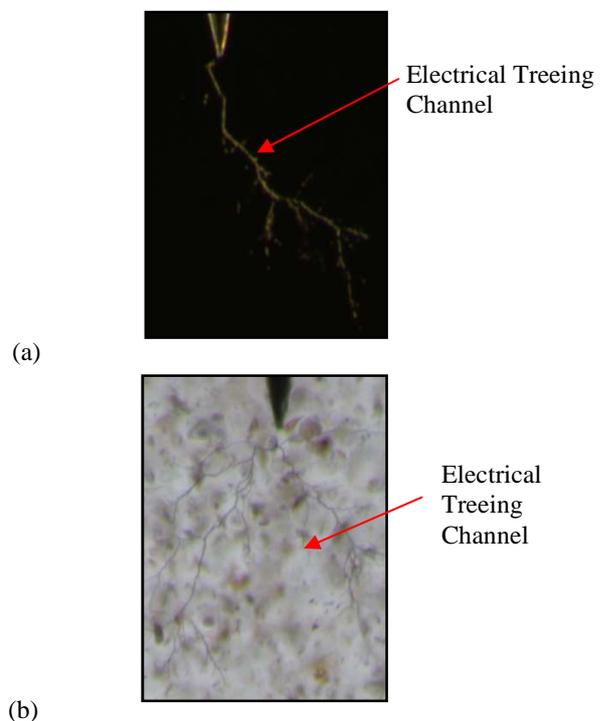
Fig. 5 Electrical tree initiation and propagation in silicone rubber (a) pure silicone rubber with tree initiated at 8.5kV and (b) silicone rubber with 1% EFB, tree initiated at 11kV
