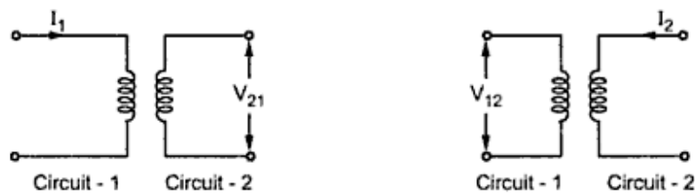
Fig 7 Representation of voltage induced in coupled circuits
