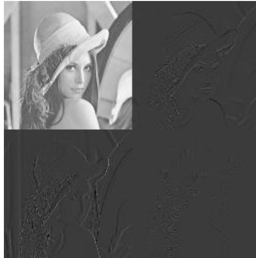
Fig11.8: Example of 4-band decomposition of an image using Daubechies 8-tap FIR filter.
