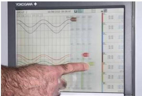
A two-point touchscreen supports swipe and pinch operations. With a single finger, an operator can swipe a trend screen and traverse across the horizontal time scale until a particular area of interest is reached (Figure 2). He or she can then use two fingers to pinch the screen in or out to compress or expand the time scale (Figure 3). This allows trend data to be examined quickly in an overview fashion, and then investigated in detail.
