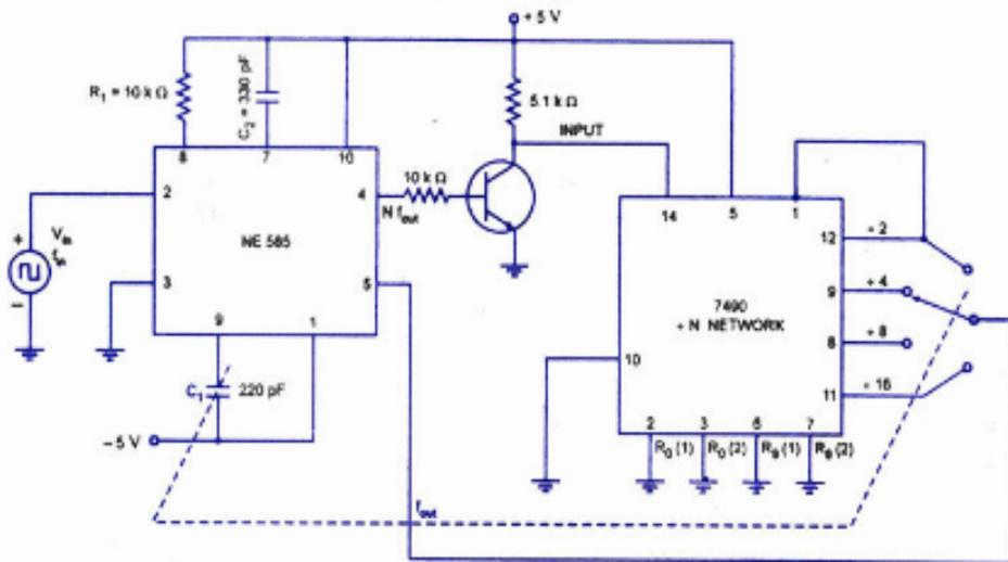
(b) Connection Diagram For Multiple Frequency Multiplier
