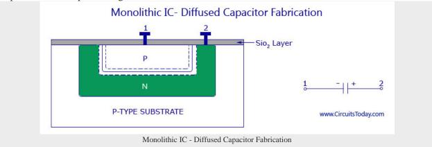
All P-N junctions have capacitance so capacitors may be produced by fabricating junctions. The amount of change in the reverse bias varies the value of junction capacitance and also the depletion width. The value may be as less as 100 picoFarads.
