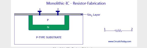
Monolithic IC - Resistor Fabrication
