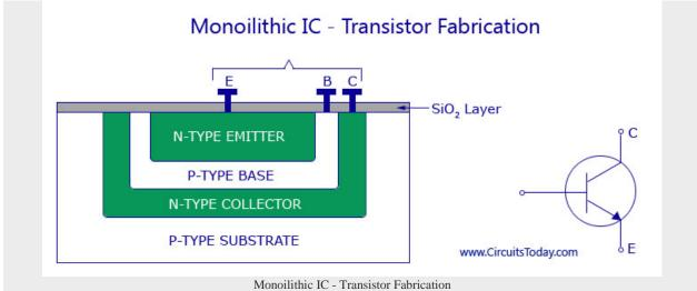
Both transistors and diodes are fabricated by using the epitaxial planar diffusion process that is explained earlier. In case of discrete transistors, the P-type substrate is considered as the collector. `But this is not possible in monolithic IC's, as all the transistors connected on one P-type substrate would have their collectors connected together. This is why separate collector regions are diffused into the substrate.
