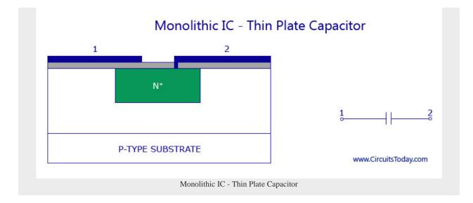
Using the silicon dioxide as a dielectric may also be a way to fabricate capacitors. One plate of the capacitors is formed by diffusing a heavily doped N-region. The other plate of the capacitor is formed by depositing a film of aluminium on the silicon dioxide dielectric on the wafer surface. For such a capacitor, a voltage of any polarity can be used, and when comparing a diffused capacitor with such a capacitor the diffused capacitor may have very small values of breakdown voltage.
