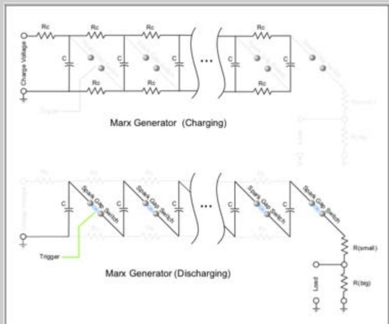
**Marx generator diagrams;** Although the left capacitor has the greatest charge rate, the generator is typically allowed to charge for a long period of time, and all capacitors eventually reach the same charge voltage.
