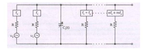
two sinusoidal signals fp and fs applied across a lossless time varying non-linear capacitance Cj (t). At the output of this varying capacitance, harmonics of the two frequencies fp and fs are generated.
