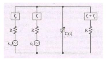
As an example, let us consider the case when the power output flow is allowed at the sum frequency fp + fs only, with all the remaining harmonics being open circuited. With the above rest ructions, the quantities 'm' and 'n' can take on values -1,0 and respectively.
