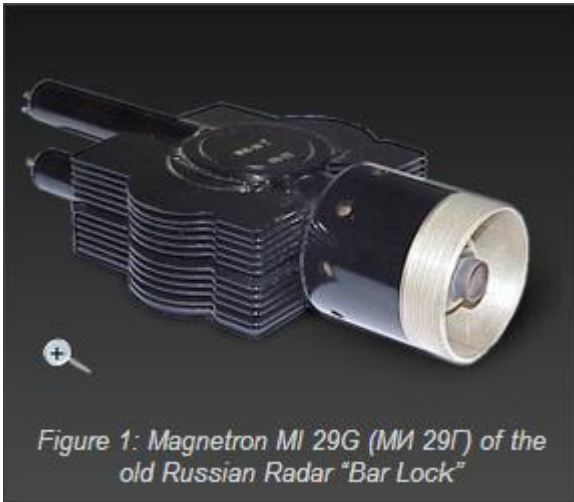
Figure 1: Magnetron MI 29G (MI 29Г) of the old Russian Radar "Bar Lock"
