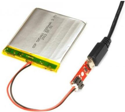
There are many low-cost chargers created to charge LiPo batteries. They commonly use USB to charge the battery. **Do not** attempt to charge a LiPos without a charger. A LiPo battery can be harmed by overcharging, so use a specifically designed LiPo charger.
