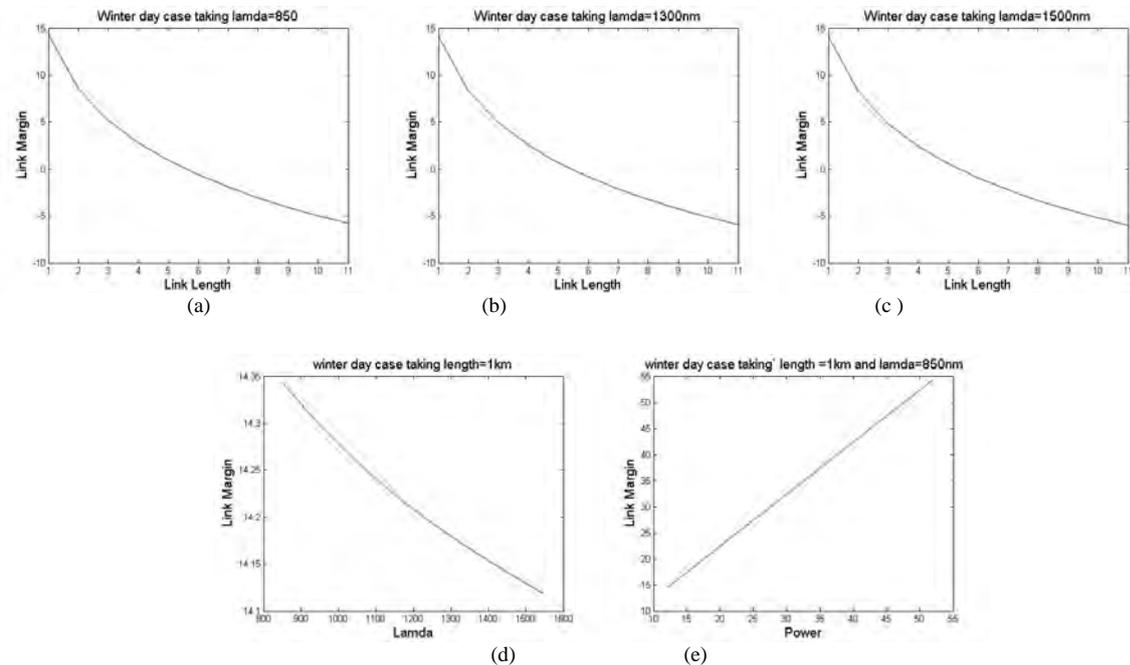
Fig3.winter conditions: (a)Link Margin v/s Link Length at  $\lambda=850\text{ nm}$ , (b)Link Margin v/s Link Length at  $\lambda=1300\text{ nm}$ , (c)Link Margin v/s Link Length at  $\lambda=1500\text{ nm}$ , (d)Link Margin v/s  $\lambda$  at 1km length, (e)Link Margin v/s Power at  $\lambda=850\text{ nm}$  with 1km length.
