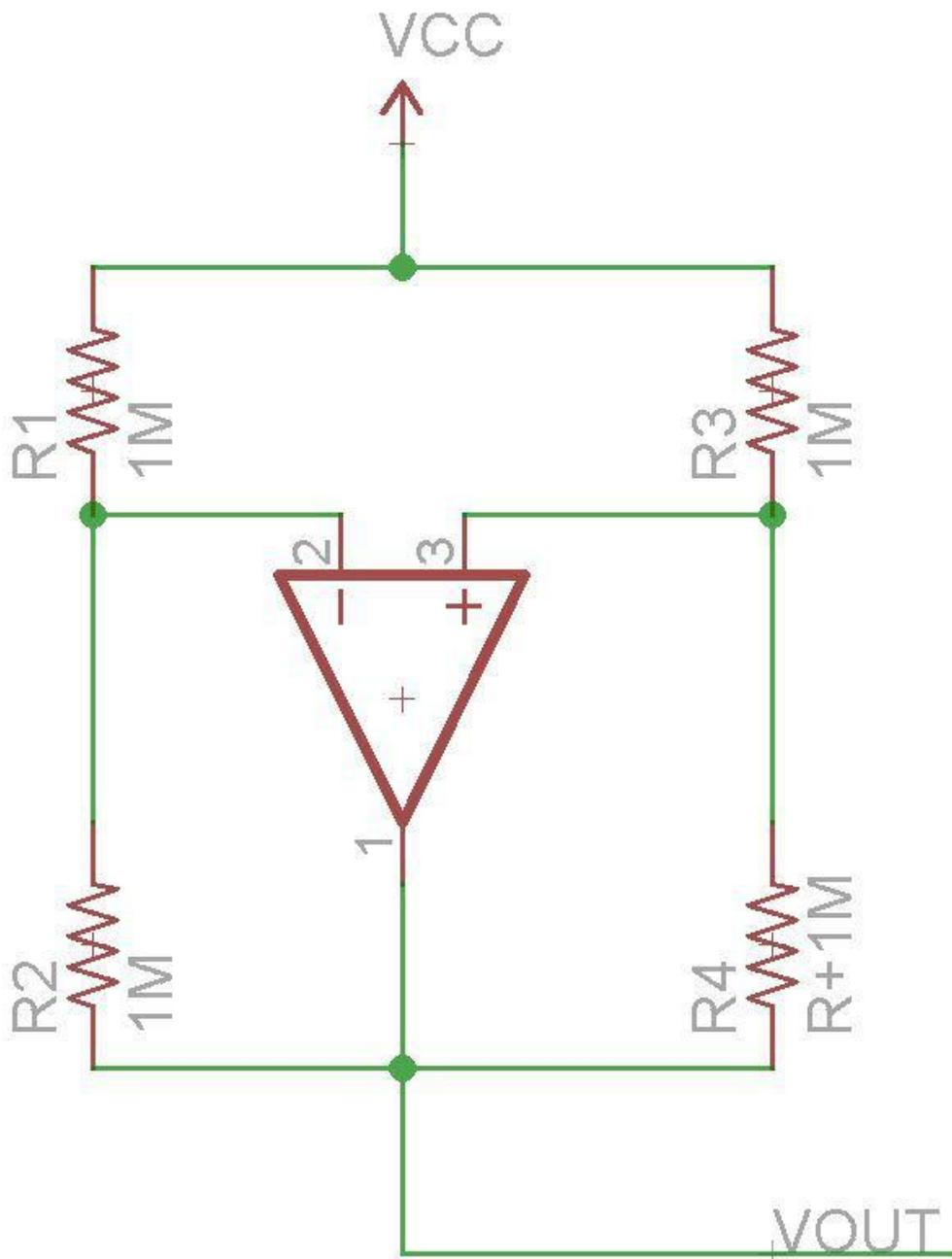
The figure above shows the linearized circuit, where the force sensor is represented as  $R_4$ , which value is change in  $R+1M$ . I won't go over the analysis, but I will show you the equation of the non-linearized circuit, and the linearized circuit. The equation below shows how the resistance of the force sensor will affect the output voltage of the circuit.
