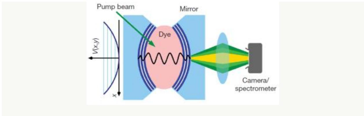
The experimental setup. A laser beam injects photons into a cavity filled with light, and a camera observes the photons coming out of the cavity. Reprinted by permission from Macmillan Publishers Ltd.
