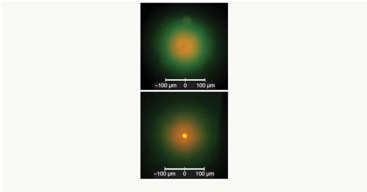
Bose-Einstein condensation of light, as observed by a camera looking at the photons from the cavity. The narrowing of the spatial distribution as the light intensity is increased (bottom image) is a tell-tale sign.
