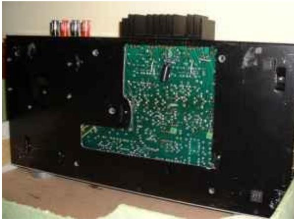
The aperture in the base of the amplifier allows access to the most often modified areas of the PCB without having to remove it from the casing.
