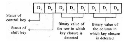
• In sensor matrix mode the condition (i.e., open/close status) of 64 switches is stored in FIFO RAM. If the condition of any of the switches changes then the 8279 asserts IRQ as high to interrupt the processor.
