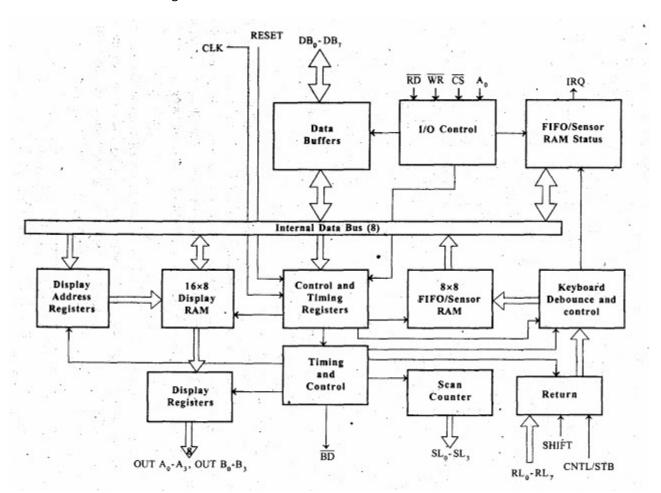
The four major sections of 8279 are keyboard, scan, display and CPU interface.
