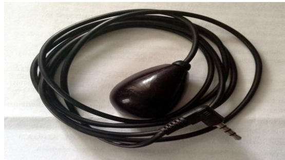
IR receiver of a SCART DVB-T tuner. Note that it has four pins instead of only two needed by a microphone.
