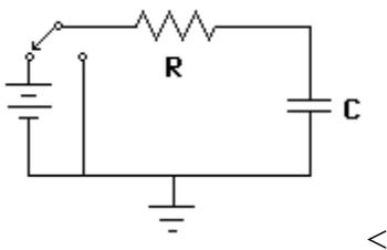
The current flow is not steady throughout this process. Starting from the discharged stage, current flows strongly at first, but slows down as the voltage across the
