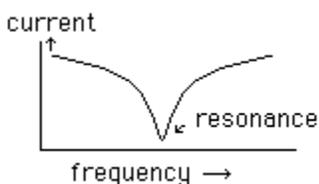
What's going on here? Well, at low frequencies, the inductor passes pretty much everything (remember, an inductor is just a wire for DC) and the capacitor blocks
