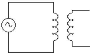
If two inductors are close together, current flowing in one will induce current in the other. Such an arrangement is called a transformer. As far as audio goes, there are three useful features of transformers:
