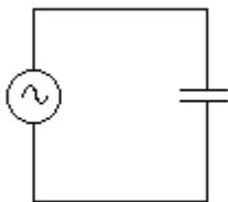
If we start with a high frequency and watch the current through the circuit, it's almost as if the capacitor weren't there at all! That's because the current is highest early in the charge cycle, and if the current source changes direction much faster than a time constant, it's always early in the charge cycle. If the frequency is reduced, the current amplitude decreases— to the point where there's nothing but a slight ripple in a steady value.
