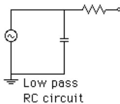
When the frequency is low, the impedance of the capacitor is high, so most current will flow through the resistor. As the frequency increases, more current is diverted through the capacitor, less to the rest of the circuit. Thus, the response is low pass. If you exchanged the capacitor and resistor, you'd have a high pass circuit.
