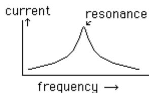
There is a magic frequency, called the resonance frequency, where plenty of current flows, but above and below resonance, there is less current. If the capacitor and the inductor are in parallel, this formula gives the impedance:
