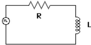
When current passes through the inductor L, a magnetic field is generated. It doesn't appear suddenly, it builds up. A magnetic field moving past a wire generates current, and a growing field is moving. In this case, it's moving past the wires of the coil itself in such a way as to oppose the incoming current, so the current flow is delayed like this:
