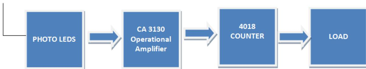
**Block Diagram of Infrared Remote Control Switch**
