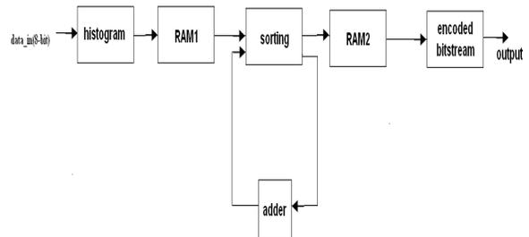
Fig 1) Block diagram for Huffman coding.
