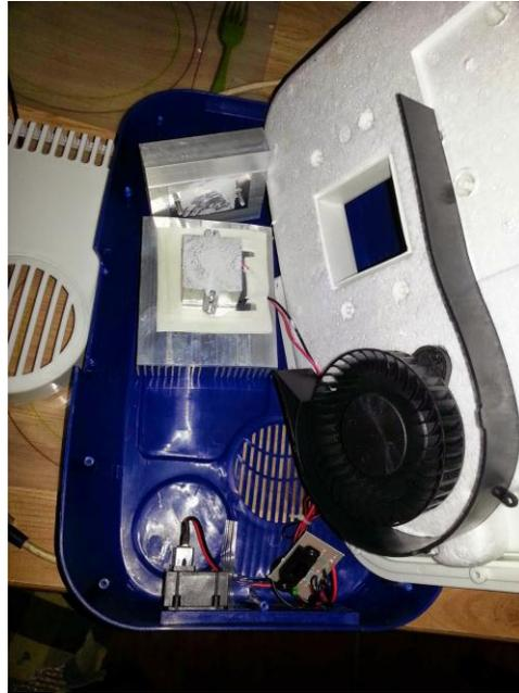
The operation could not be easier; carries no power control ; it's just a switch that directly feeds the two small fan motors and peltier cell, plus a small diode with a resistor to lower the voltage.
