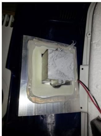
**Now we only go in reverse and mount it as it was** , being careful that the screws are firmly fixed sinks, because if the cell does not make proper contact with the heatsink, it would spoil quickly and cool down very little.
