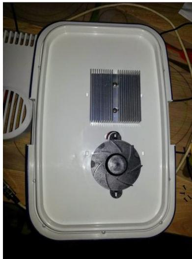
We can lift, and at the bottom we see the heat sink; peltier cell medium set with white heat conductive paste, then a billet aluminum to overcome the isolation of styrofoam to the other side, which is attached cooler cools the portion smaller.
