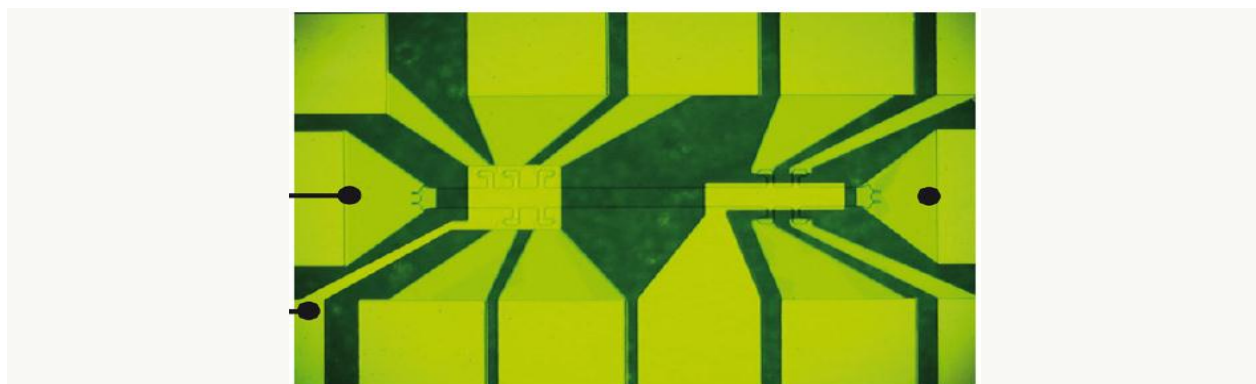
Photo of the electronic device used to measure the high electron mobility in ZnO. Reprinted by permission from Macmillan Publishers Ltd. Nature Materials (2010). doi:10.1038/nmat2874
