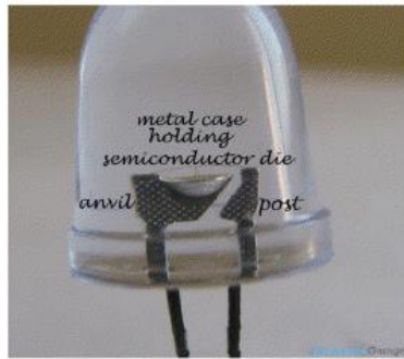
Figure 4 Close view of metal case holding semiconductor die
