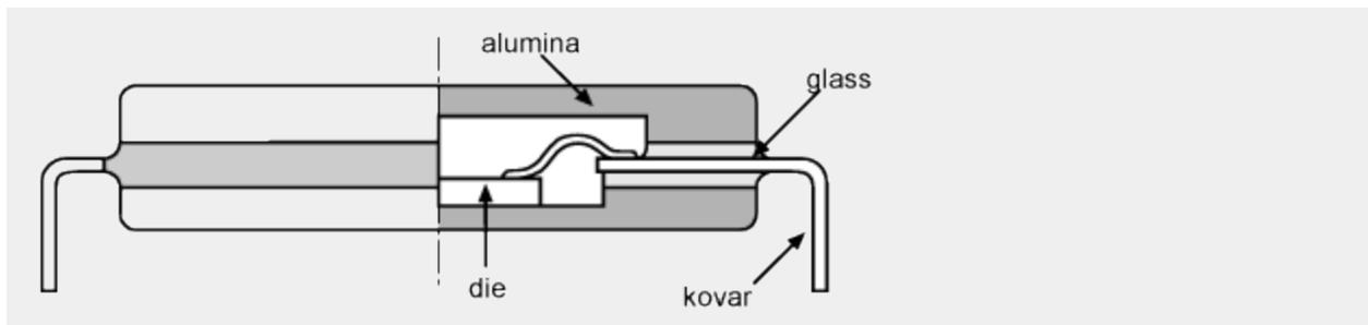
**Figure 10: Ceramic package constructions: side-braze (left) and chip carrier (right)**
