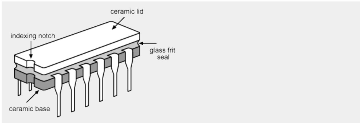
**Figure 9: The flat-pack construction**
