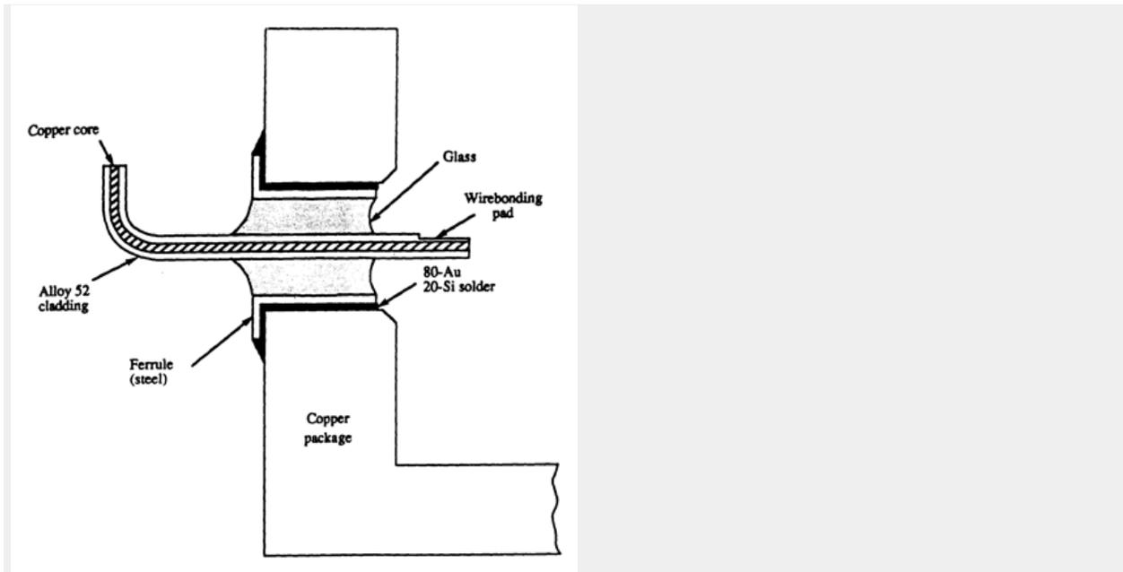
The length of the glass path between contact and outer body determines the resistance of the seal to arcing at high voltages. For matched seals, voltage breakdown is in the order of 40VAC for each 25µm of path.
