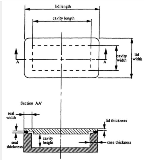
Figure 7: Typical covers used in hermetic sealing of hybrid packages
