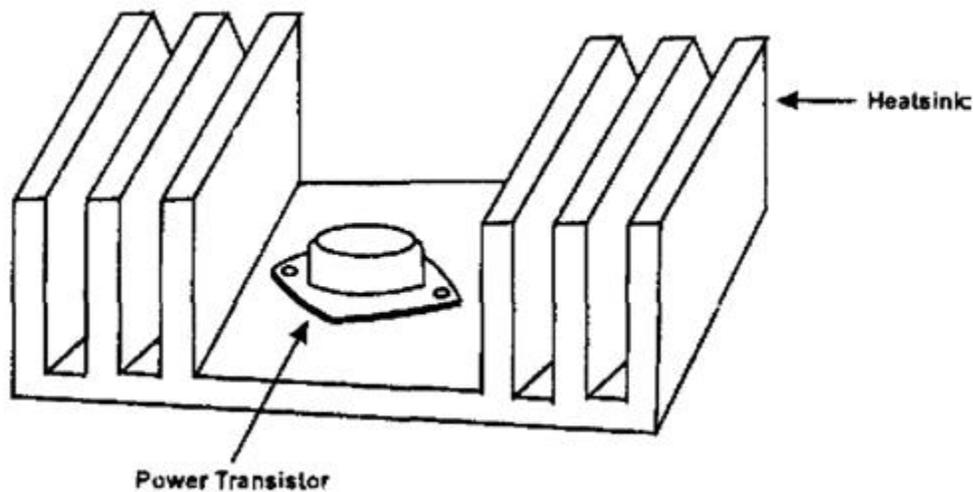
Fig shows a heat sink. The heat now radiate more quickly because of in creased surface area.
