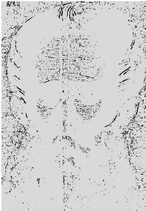
Fig. 5. Thresholded output of the top-hat transform (threshold value: 19). A number of brush strokes (hair, number in the upper left corner) have been misidentified as cracks.
