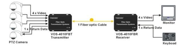
If camera control is used then the fibre optic link interface electronics must be compatible with
