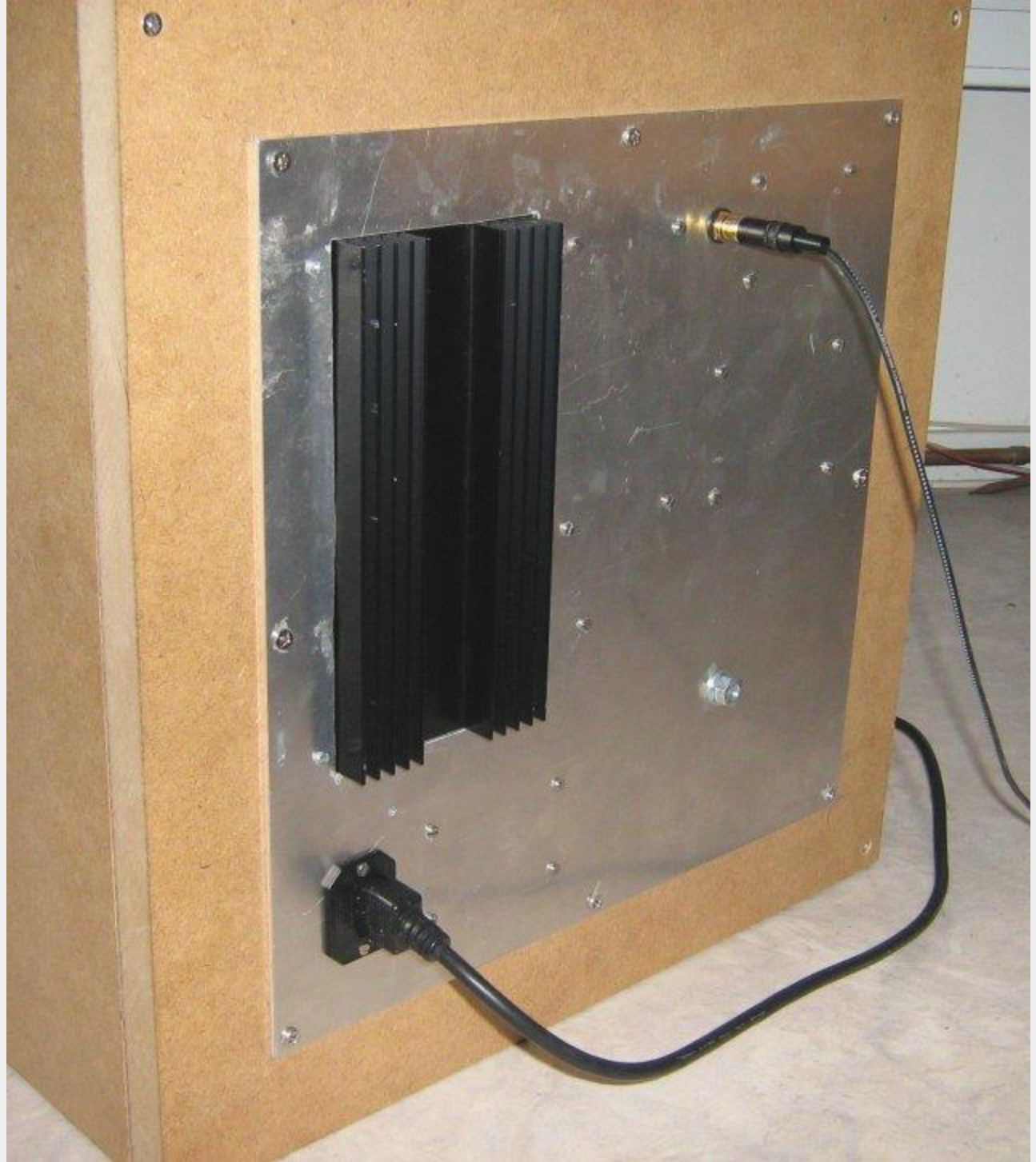
The back of the unit. Small heatsink huh? It suffices for normal program material.
