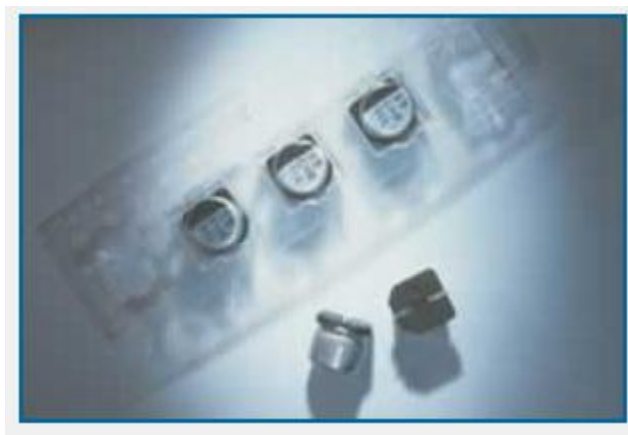
Aluminium electrolytic capacitors in a surface mount package
