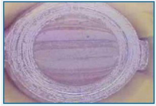
Figure 6: Macroscopic image showing fatigue beachmarks (x6.5)
