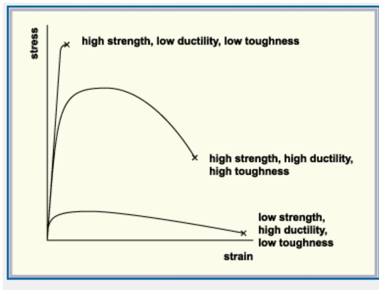
Figure 1: Typical stress-strain curves
