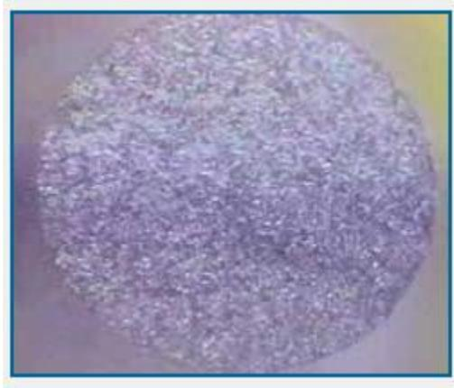
Figure 4: Macroscopic image of a brittle fracture (x6.5)
