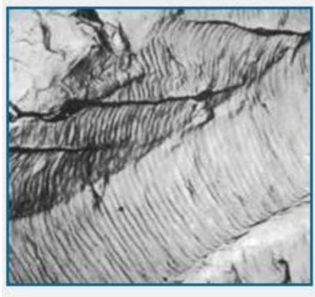
Figure 7: Scanning electron microscope image of fatigue striations (x1000)
