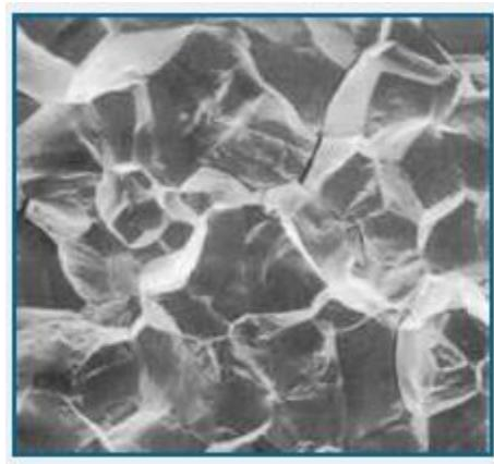
Figure 5: Microscopic image of intergranular brittle fracture (x1000)
