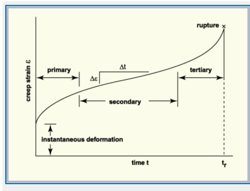
Figure 9: Creep strain versus time graph
