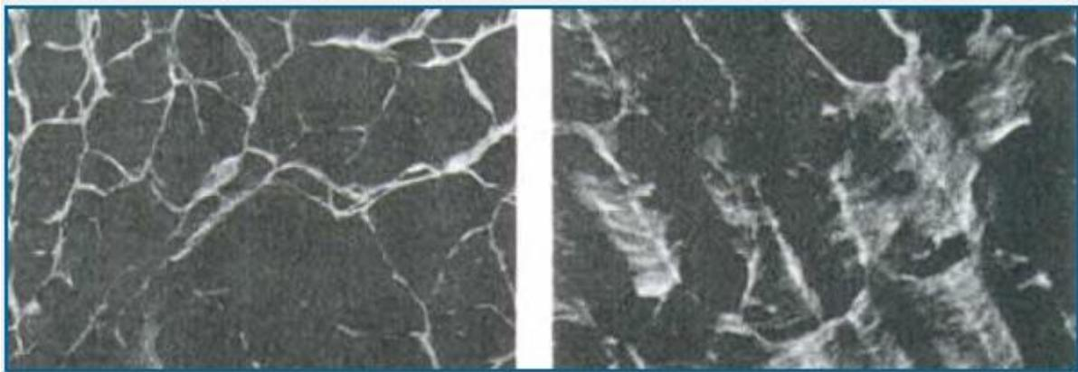
Figure 3: Microscopic images of ductile fractures (x1000)
