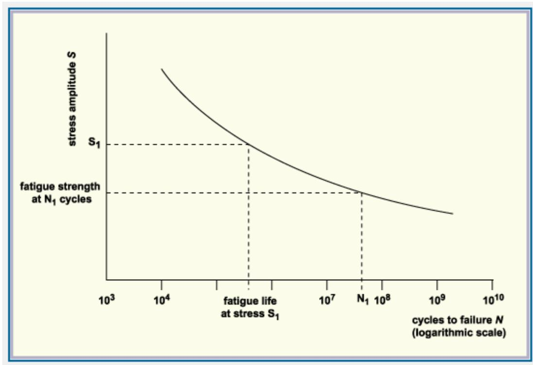
Figure 8: S-N curve for non-ferrous materials such as solders
