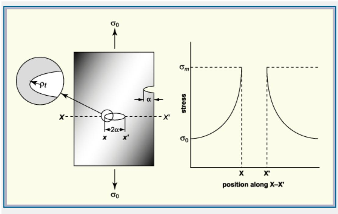
Figure 10: Schematic representation of stress-raising defect
